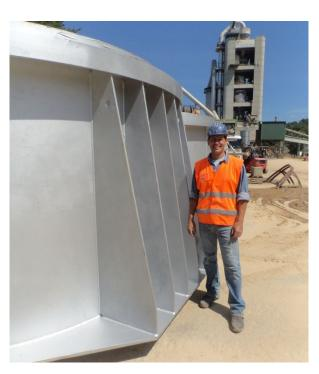
The latest modification applies the replacement of four cyclones and all appropriate input and output ducts to the raw mill and was realised in 2015. The result was a reduction of dust by 66%, a reduced power consumption and a low pressure drop of the cyclones (6,1 mbar) as well as an excellent seperation efficiency of 95%.
