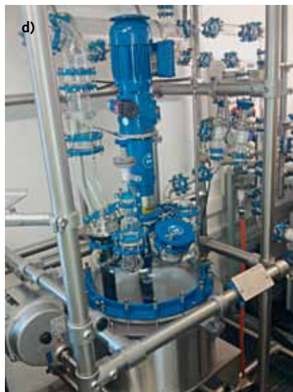
5 Mixer (a), filter press (b) and sedimenter (c), crystallizer (d) and drying ovens (e) installed in the process container
