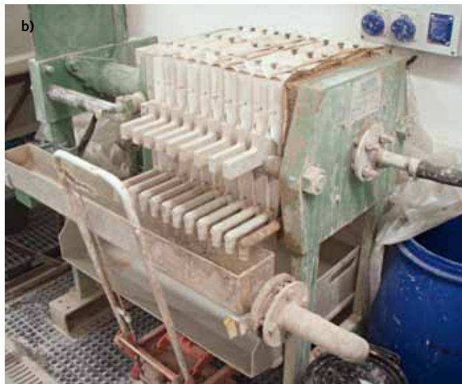
5 Mixer (a), filter press (b) and sedimenter (c), crystallizer (d) and drying ovens (e) installed in the process container
