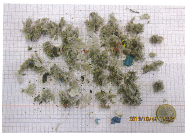
Figure 5. Relation of the mill's output material to a coin.
