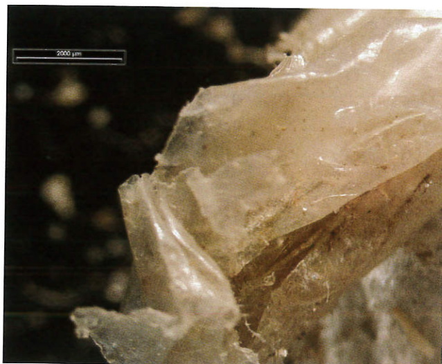
Figure 4. Solid AF produced by a conventional shredder.
