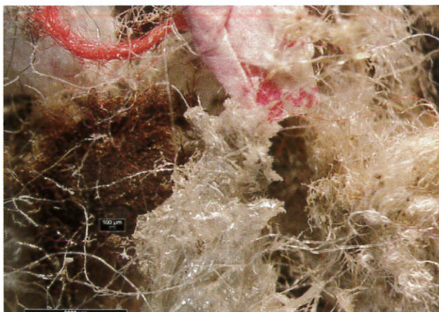
Figure 3. Solid AF produced by the Rocket Mill.
