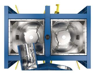
The mill consists of two robustly-designed grinding chambers, each of which is equipped with four to eight horizontally rotating chains and perforated screens.
